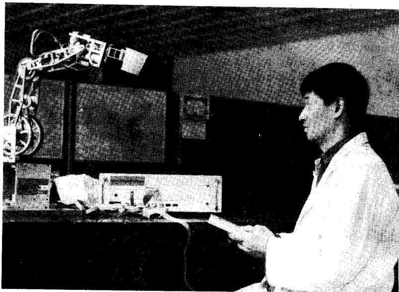
China's first robot programmed to perform teaching functions. The robot, developed by the Shanghai Meters Plant, is also able to make 360-degree turns, while its manipulator arm can pick things up, write and draw.
